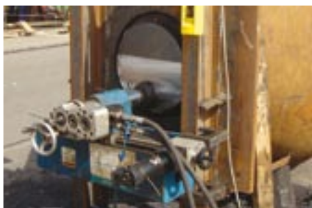
Special setup for machining the spuds
